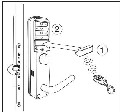
When installing a remote control, assure that the receiver is inserted on the inside and that this is done before the batteries are inserted.
